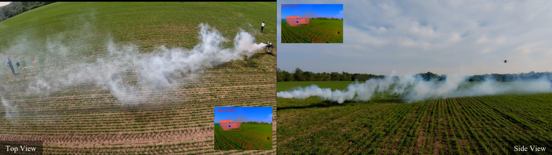
Drone autonomously tracking real smoke plume using PID/DRL [red bounding box: drone location]
